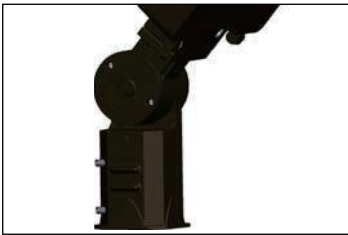
Slipfitter Mount An optional case aluminum mast arm adapter secures fixture head to nominal 2-3/8"O.D. horizontal steel tenon arm.
